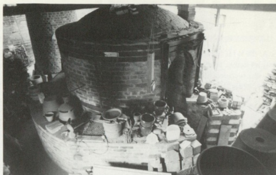
Jonathan Garratt. Round downdraught kiln, 7ft across by 7ft high – halfway up dome, four Bourry fireboxes, chimney 25ft tall – 7ft across outside at ground level
